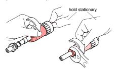
6 Plug in the connector and secure it with the union nut.
